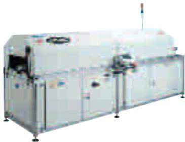
The IR2000 from PVA offers complete infrared heat capabilities in four foot or eight foot curing lengths. Single or double-sided processing is available with maximum IR panel temperatures reaching 260-degrees Celsius (500-degrees Fahrenheit). Each heating zone measures 24" (610 mm) in width and can be
